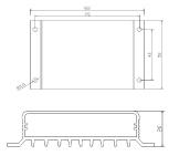
$\label{eq:linear} \begin{array}{l} \text{I.The size of CM100-LI} & \text{is as follows:} \\ \text{Boundary dimension: } 82 \times 100 \times 20(\text{mm}) \\ \text{Installation dimension: } 86 \times 75(\text{mm}) \\ \text{Installation aperture: } 3.5(\text{mm}) \\ \text{2.The size of CM50-LI and CM20-LI:} \\ \text{Boundary dimension: } 82 \times 58 \times 20(\text{mm}) \\ \text{Installation dimension: } 43 \times 75(\text{mm}) \\ \text{Installation aperture: } 3.5(\text{mm}) \end{array}$
