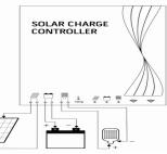
Connection sequence: Please connect the storage battery first, then connect the load, last is the solar panel. Pay attention to the "+" and "-" in case of reverse connection.
